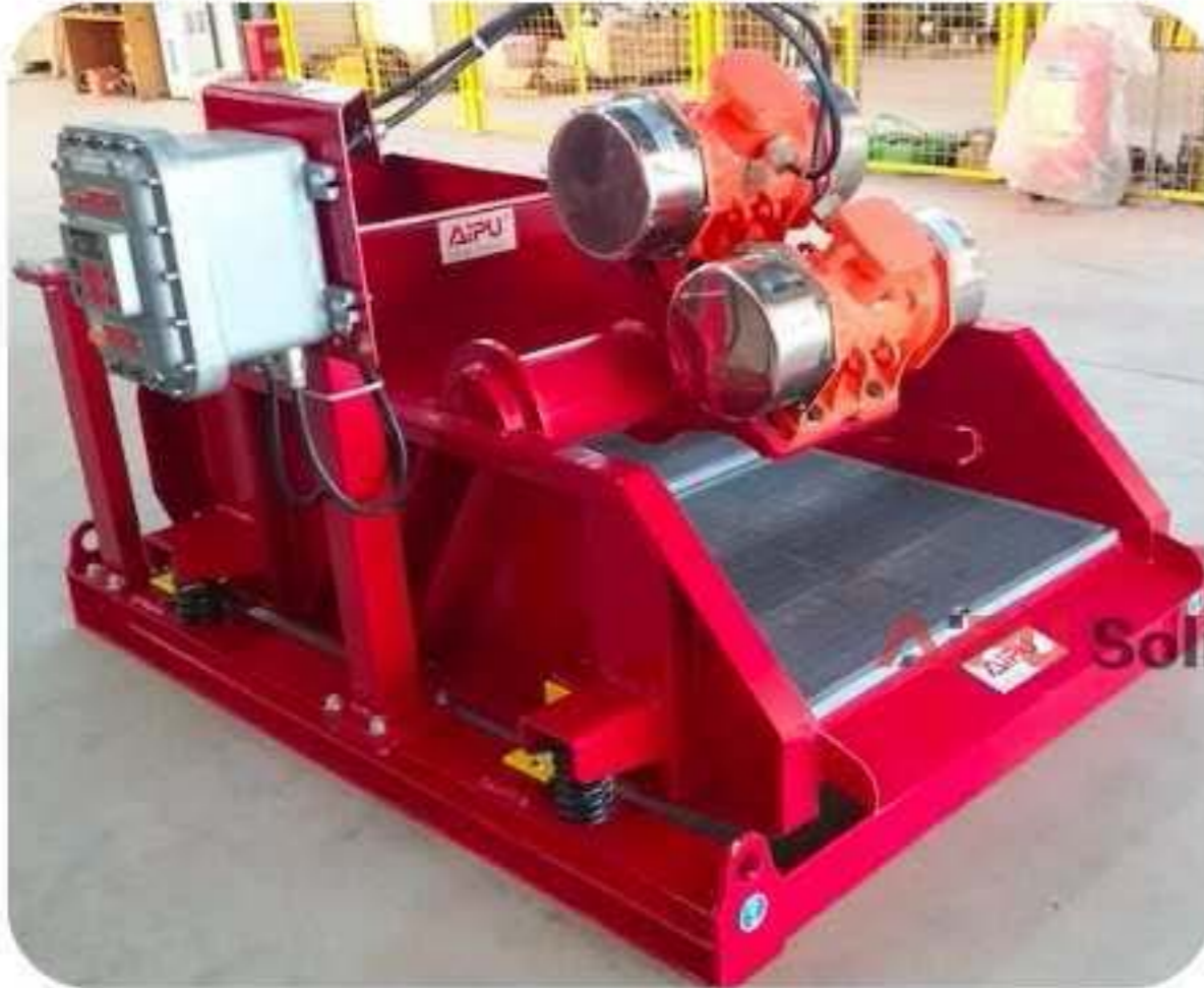
Mini shale shaker for oil sludge treatment
