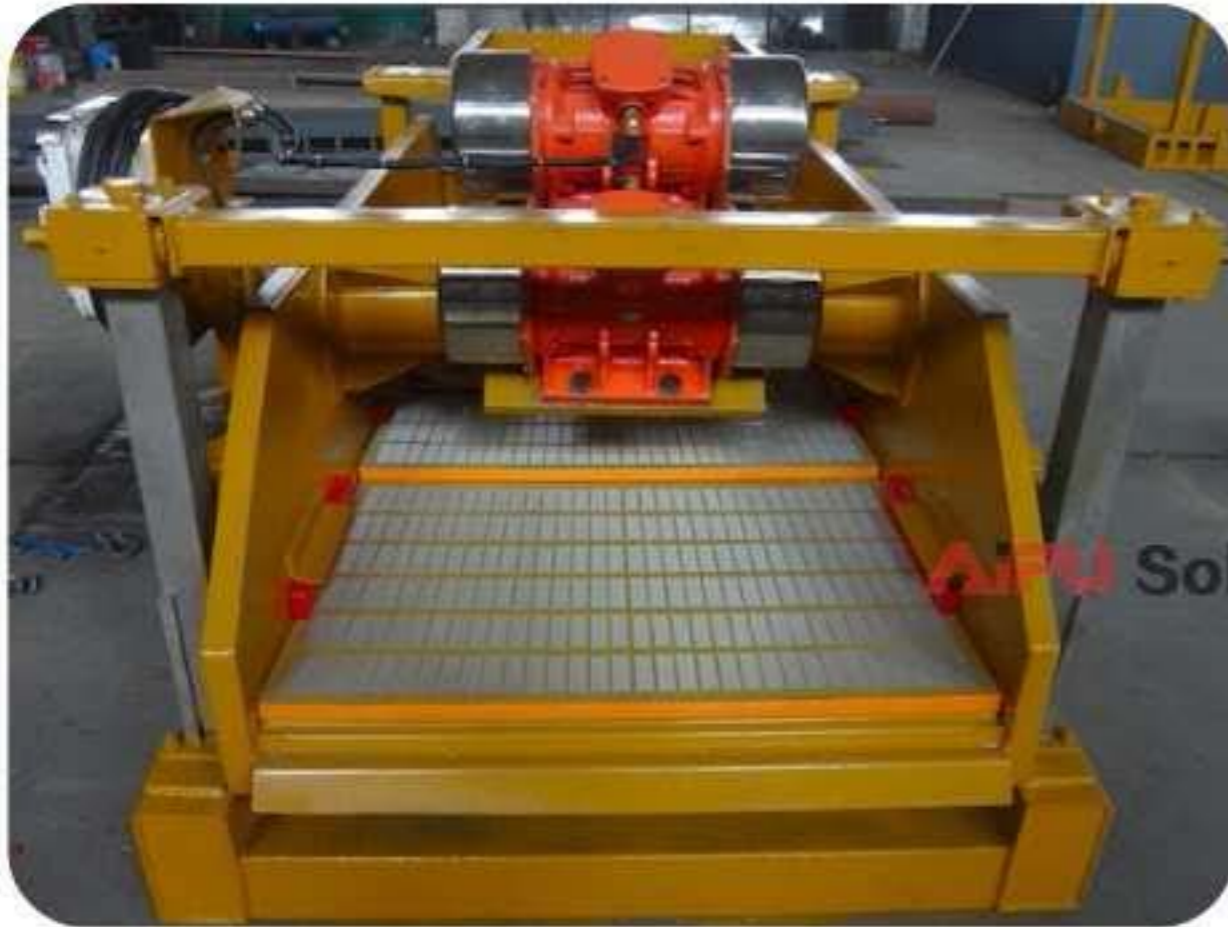
Aipu shale shaker with composite frame screen
