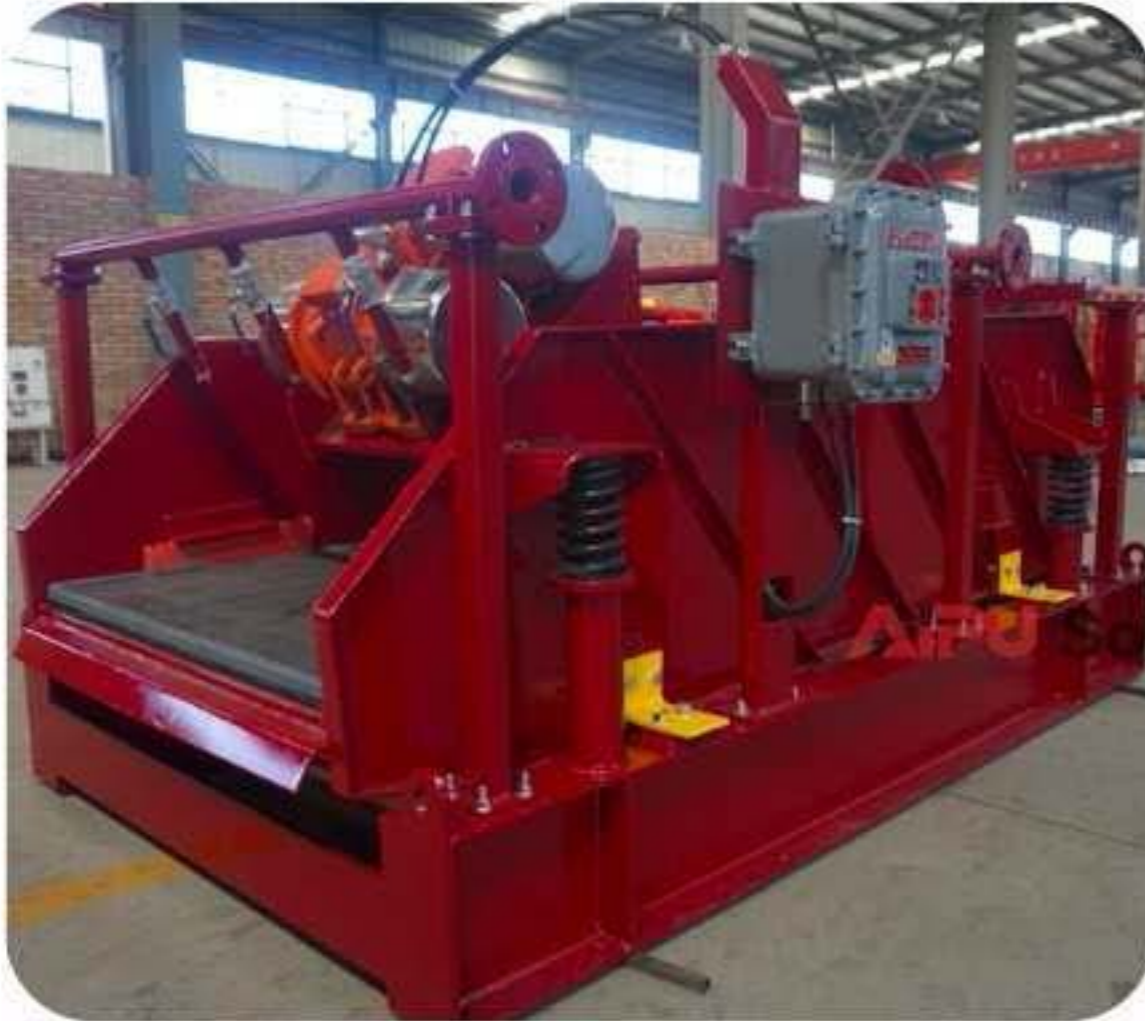
Shale shaker with flush pipe
