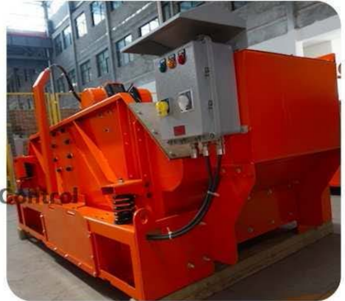
Dual motion shale shaker painted orange
